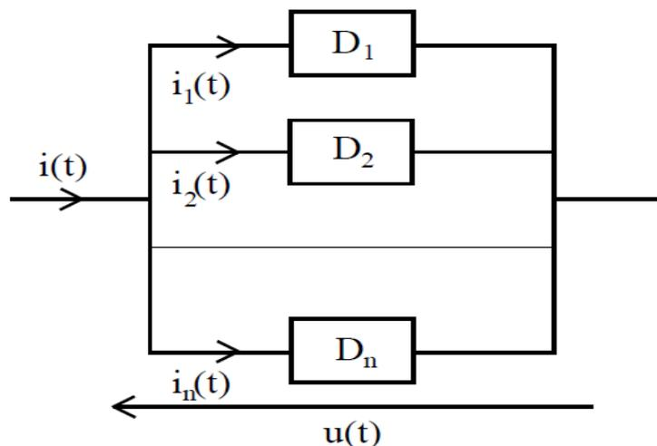
$$i(t) = \sum_k i_k(t) \quad \text{et} \quad u_k(t) = u(t), \quad \forall k$$
